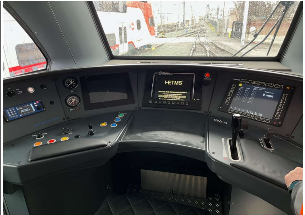
BROAD VIEW AHEAD FOR THE ENGINEER – Clear line of sight with 180-degree view of the tracks and train operations shown on multiple screens.
